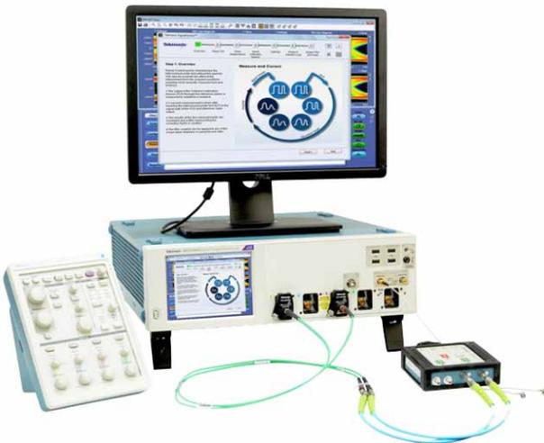
SignalCorrect allows quick characterization of cables, fixtures and other types of interconnects using the TCS70902 fast step source and the response captured on a DPO7000SX Series real-time oscilloscope.
