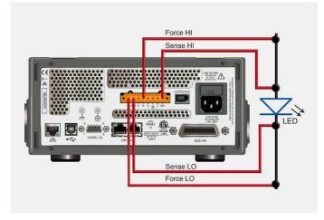
FIGURE 5. 2461 4-wire rear-panel connections to an LED.
