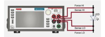
**Figure 5** shows the rear-panel connections. You can make these connections with either the 2460-KIT Screw Terminal Connector Kit (included with the 2461) or a 2460-BAN Banana Test Leads/Adapter Cable with appropriate cabling.
