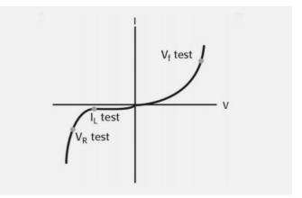
FIGURE 6. Typical HBLED DC I-V curve and test points for manufacturing tests (not to scale).
