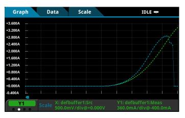
FIGURE 2. Two I-V sweeps run on the same HBLED. The green curve is a pulse I-V sweep. The blue curve is a traditional I-V sweep that led to overheating and
