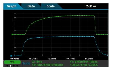
FIGURE 8. Using the 2461's digitizing A/D convertor to show the Vf pulse response. The forced voltage waveform is shown in blue and the measured current waveform is shown in green.
