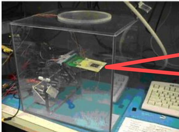
Figure 4. One Cubic Foot Still Air Chamber
