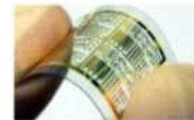
Flexible carbon nanotube integrated circuit
