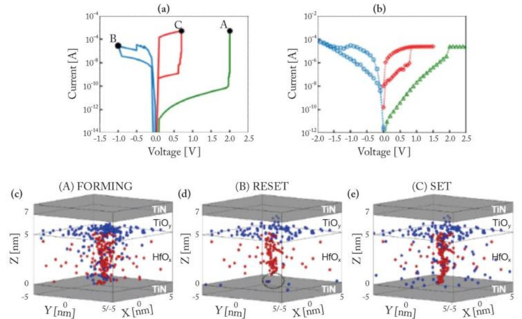
Figure 3.8: Simulated forming-reset-set process for a TiN/Ti/HfO<sub>x</sub>/TiN RRAM device using the 3D KMC simulator. (a) Simulated (b) experimental I-V characteristics. V<sub>o</sub> (red) and O<sup>2-</sup> (blue) distributions at the end of (c) forming, (d) reset, and (e) set operations. Adapted from [64].
