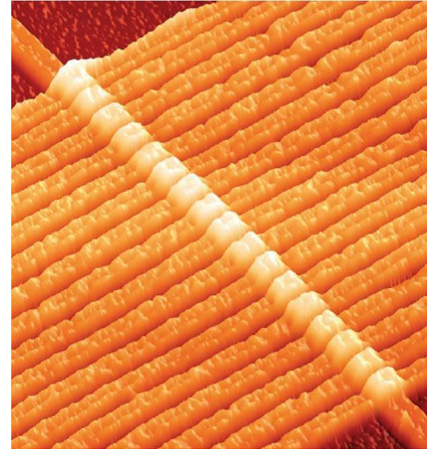
**Crossbar Architecture:** A memristor's structure, shown here in a scanning tunneling microscope image, will enable dense, stable computer memories. *Image: R. Stanley Williams/HP Labs*
