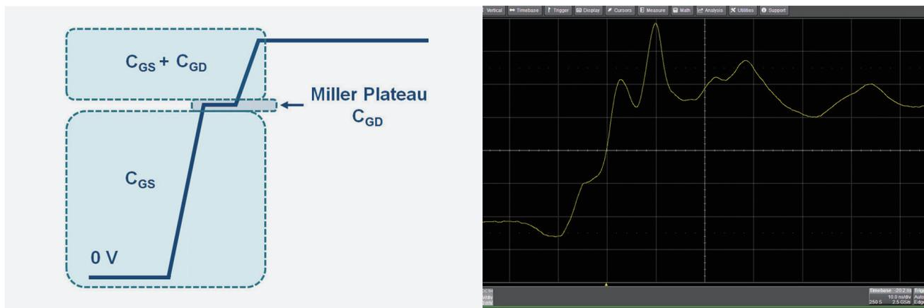
图 4: Comparison of LeCroy's DA1855A High-Side  $V_{GS}$  Output to Ideal.
