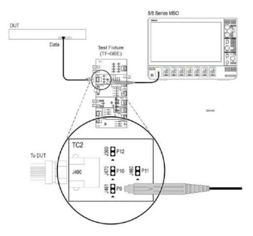
1000BASE-T Distortion (without Disturber; without clock)
