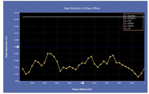
Transmitter Distortion without TX\_CLK
