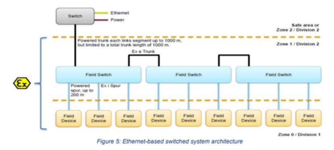
In order to reduce installation costs and cabling effort, the connection to the field is realized by a *Trunk* and *Spurs* as depicted in both Figure 5 and Figure 6. The Trunk and Spur provide sufficient bandwidth for
