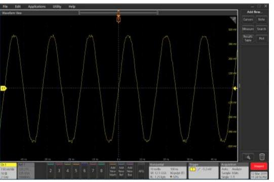
1000BASE-T Test Mode-2 waveform
