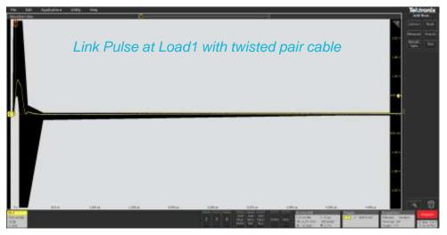
A LTP should be bounded between  $\pm 3.1$  V with a width of no greater than 42 Bit Times (4200 ns)
