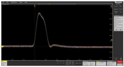
10BASE-T Link test pulse, transmitted every 16ms ±8ms and is ~60ns to ~200ns wide
