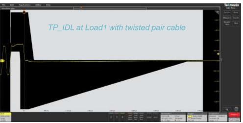
The Start of Idle (SOI or Start of TP\_IDL) occurs at the end of a packet and shall always begin with a positive waveform.
