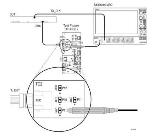
1000BASE-T Distortion (without Disturber; with clock)
