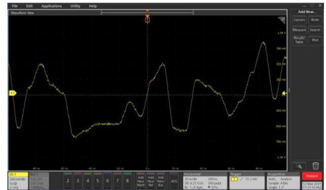
1000BASE-T Test Mode-4 waveform
