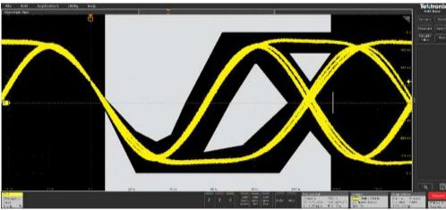
MAU Template test – Internal (Top) and Inverted (Bottom)
