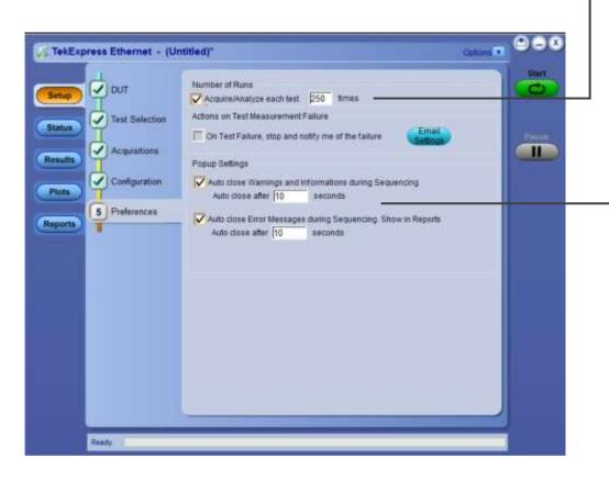
This option enables multiple test runs in a single execution. Use this option to check for repeatability of test results
