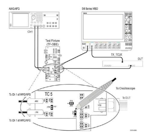
1000BASE-T Distortion (with Disturber; with clock)
