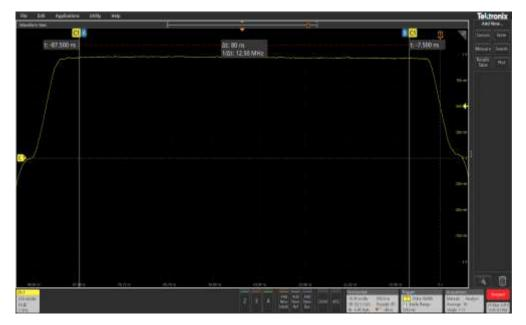
Amplitude tests performed on long run of logic high levels
