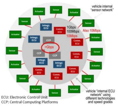
Figure 7: Automotive Ethernet architecture concept
