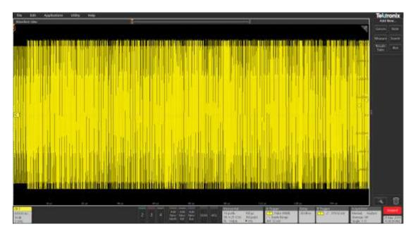
The peak differential voltage a device transmits shall be between 2.2V and 2.8V. This means the height of a frame should never be below -2.8 volts and above +2.8volts or should never be below 2.2 volts and above -2.2 volts.
