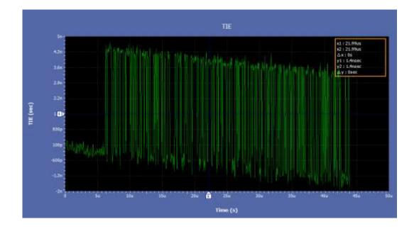
Jitter is measured at the 8 and 8.5 Bit times with and without the TPM present. With out the TPM a zero crossing should occur  $\pm 20$ ns at the 8 and 8.5 BT. With the TPM a zero crossing should occur  $\pm 11$  ns at the 8 and 8.5 BT.
