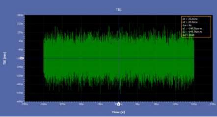
Positive and Negative Jitter measured using TIE Jitter Method
