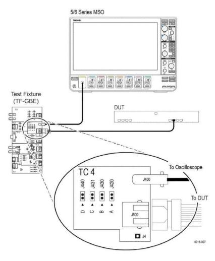
1000 BASE-T Common Mode Voltage Test Setup
