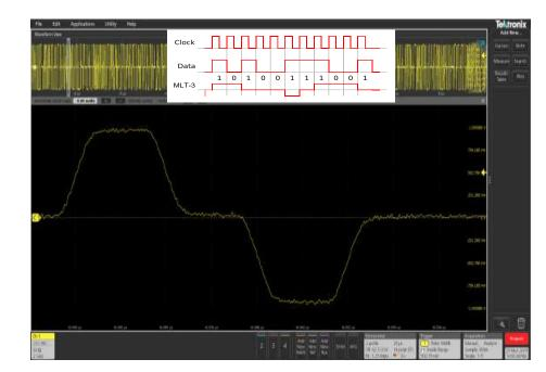
100 BASE-TX Multi-Level Transmit 3 (MLT-3) Line Encoding
