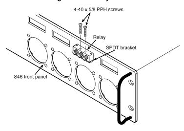
Figure 1: S46 relay installation
