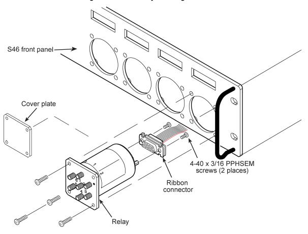
Figure 3: 18 GHz relay A through D installation
