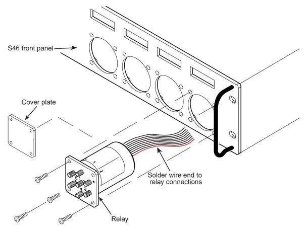
Figure 4: 26.5 and 40 GHz relay A through D installation
