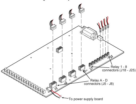
Figure 2: S46 relay connector locations
