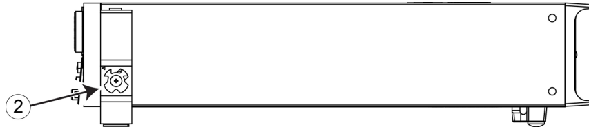
Figure 8: Remove mounting ears
