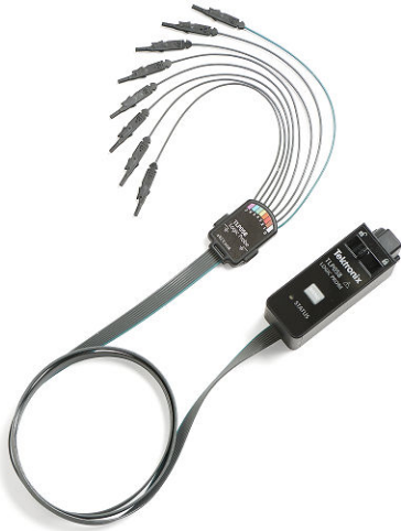
Figure 3: The TLP058 provides eight high performance digital inputs. Connect as many TLP058 probes as you like, enabling up to a maximum of 64 digital channels.
