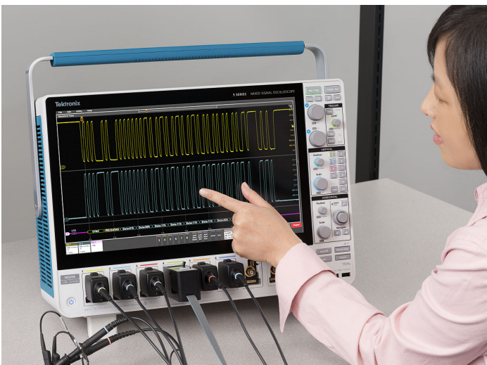
Figure 9: Interact with the capacitive touch display in the same way you do on your phones and tablets.
