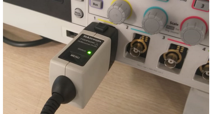
Figure 9: TekVPI probes communicate scale settings, ranges, and status to the TBS2000B.
