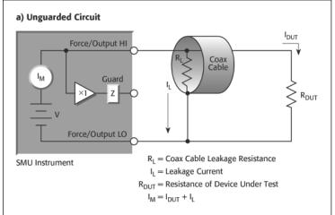
The coax cable's signal to lo resistance causes a parallel current path that slows down settling times and limits the low current resolution of the system.
