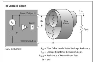
The extra shield in the triax cable works with the driven guard in the SMU instrument to virtually eliminate the parallel current path. This enables faster settling times and better measurement resolution.
