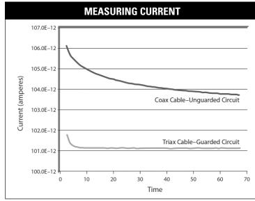
Triax cables enable faster settling times and better resolution when sourcing or measuring.
