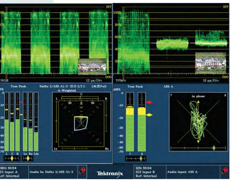
selected. For the two audio inputs a Lissajous display was selected to show the interaction of the phase of the two channels
