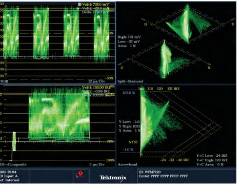
center of the display represents the lower black region of the signal and the upper and lower points of the diamond represent the white limits for the signal. A straight line from the center to the outer point of the diamond indicates a correctly balanced luma only signal. The gamut limits are adjustable within the configuration menu. In this case the EBU-R103 limits were applied.
