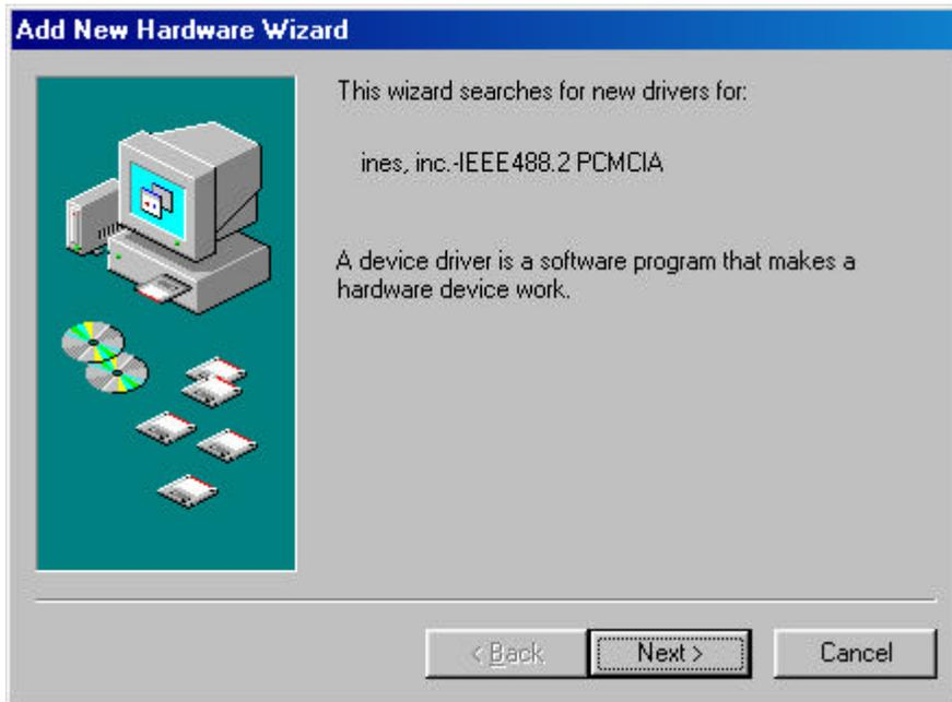
Since the CD contains an inf file for Windows to use, the automatic search for a driver works well so long as the CD drive is included as a source that should be searched. Click Next button.
