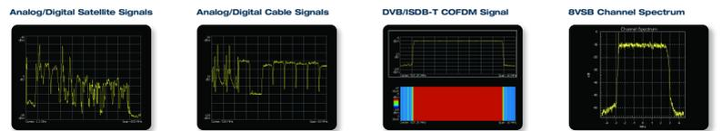
Ku-Band (10-12 GHz) and C-Band (4-6 GHz) satellite feeds are downconverted to L-Band (950-2250 MHz) using a Low Noise Block (LNB). The L-Band example above shows several analog NTSC transponders along with several MPEG-2 QPSK transponders.
