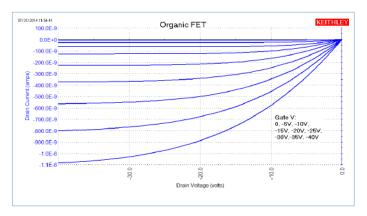
Figure 16. Transfer characteristics of OFET measured by Model 4200-SCS Parameter Analyzer. Note: OFET courtesy of Kent State University.
