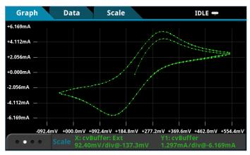
Figure 3. Voltammogram generated on 2450 graphical display.
