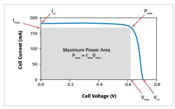
Figure 9. Typical forward bias I-V curve of a photovoltaic cell.
