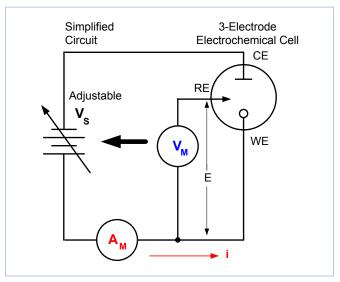
Figure 1. Simplified measurement circuit for performing cyclic voltammetry.
