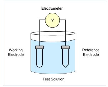
Figure 7. Electrometer measuring potential difference between two electrodes.
