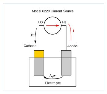
Figure 17. Electroplating circuit using a constant current source.
