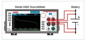
Figure 12. Results of discharging battery shown on graphical display of Model 2460 SourceMeter SMU instrument.
