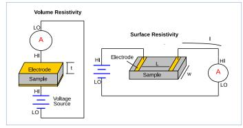
Figure 6. Volume and surface resistivity measurement diagrams.
