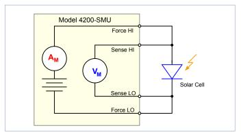
Figure 10. A solar cell connected to a Model 4200-SMU Parameter Analyzer.
