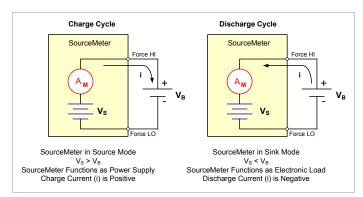
Figure 13. Charge and discharge circuit diagrams.
