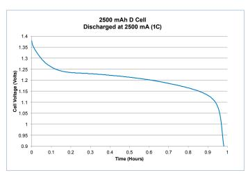
Figure 14. Discharge characteristics of 2500 mAh D cell battery using Model 2460.
