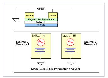
Figure 15. Model 4200-SCS parameter analyzer for organic FET I-V characterization.
