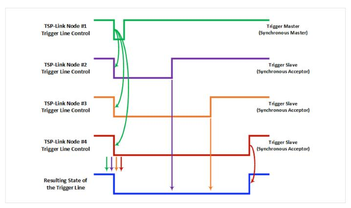
Figure 9. How the Synchronous Master and Acceptor trigger modes work.
