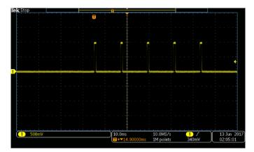
Figure 17. Voltage profile for 100 mA current pulses with a resistor.
