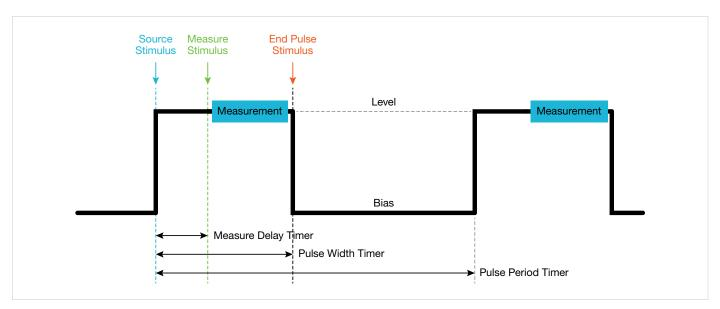
Figure 5. Laser diode and photodiode pulse I-V sweep pulse diagram.
