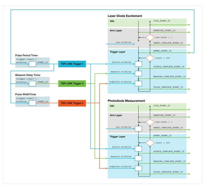
Figure 7. Modified trigger model for sharing trigger signals with remote nodes.
