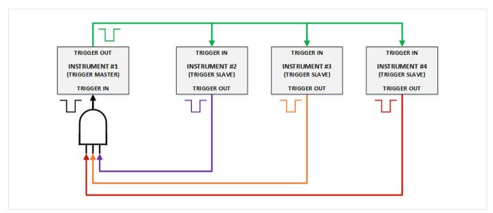
Figure 8. Closed loop control scheme using conventional triggering.
