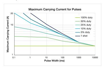
Figure 16. Maximum current carrying capacity and pulse width.
