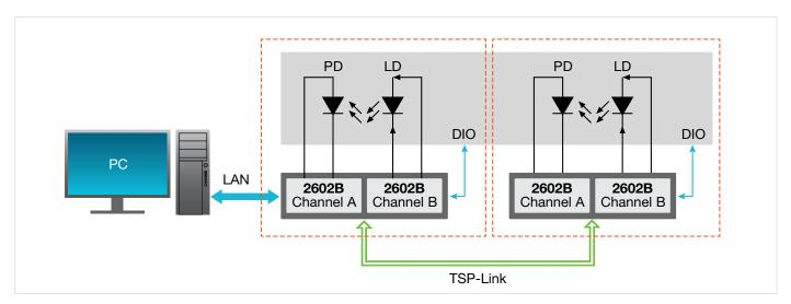
Figure 6. TSP-Link enabled multi-channel system.
