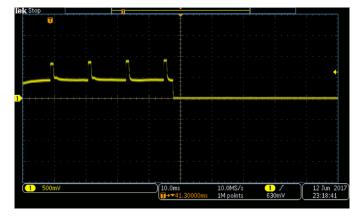
Figure 18. Voltage profile for 100 mA current pulses with a diode or laser diode.
