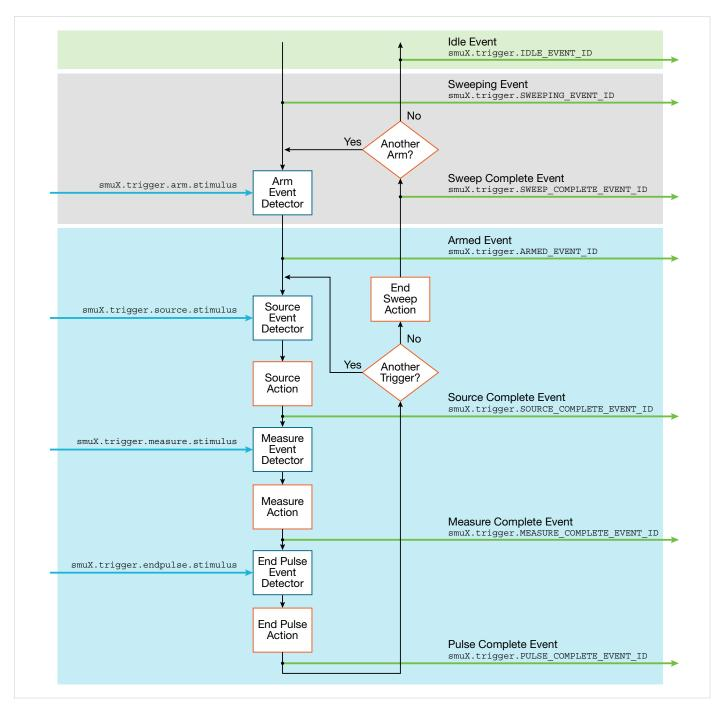
Figure 3. Flow chart for synchronous trigger model.
