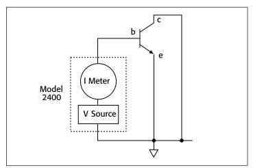
Figure 4b. Base leakage current
