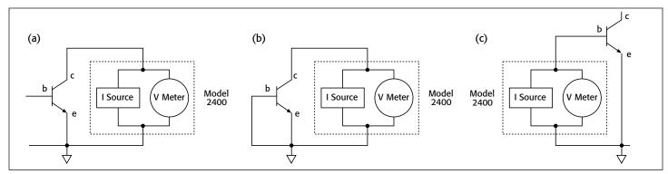
Figure 3a. Collector-emitter breakdown with base open; 3b. Collector-emitter breakdown with base shorted; 3c. Emitter-base breakdown with collector open
