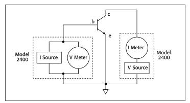
Figure 5a. DC gain measurement setup
