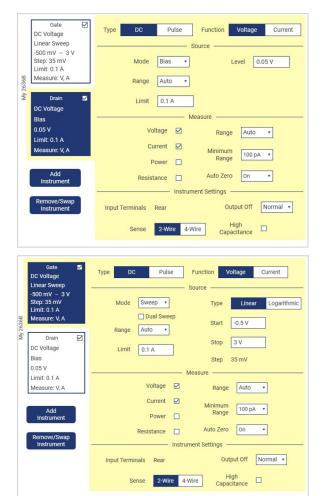
Figure 4. Drain (top) and gate (bottom) settings for transfer measurement in KickStart.
